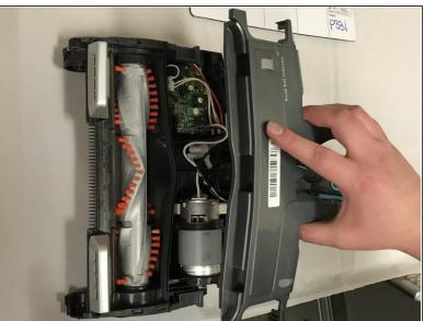
Turn over the machine and lift the top casing off.
