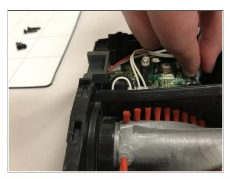
Remove large white plastic plug using your fingers and/or long nose pliers.
