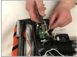
Remove the caps from the red, black and yellow wires to expose the three metal clamps.
