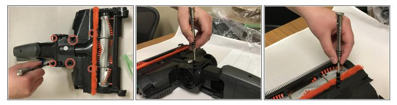
• Unscrew the six 18.7mm screws in the bottom casing using a T20 screwdriver.
