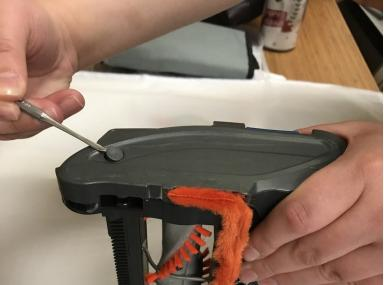
Gently pry the circular screw cover off of the side of the casing with the shoe print mark on it with the small metal spudger.
