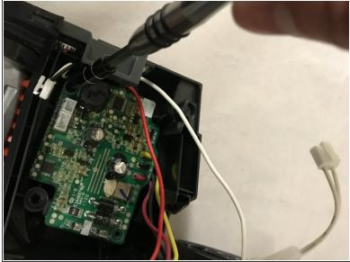
Unscrew the two 11.8mm screws in the motherboard using a T10 screwdriver.
