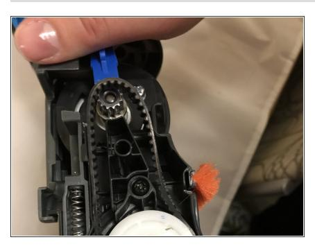
Use the large plastic opening tool to pry the rubber brushroll band towards you until the rubber brush roll band comes off of the small metal gear.
