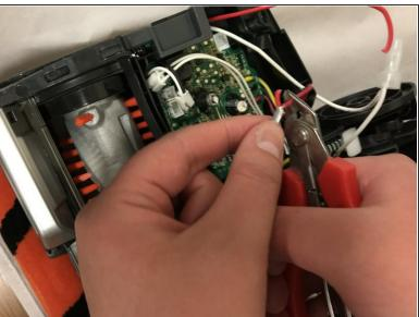
Cut the red wires extending beneath the metal clamp, right below the metal clamp holding the two wires together. Repeat process for black and yellow wires.
