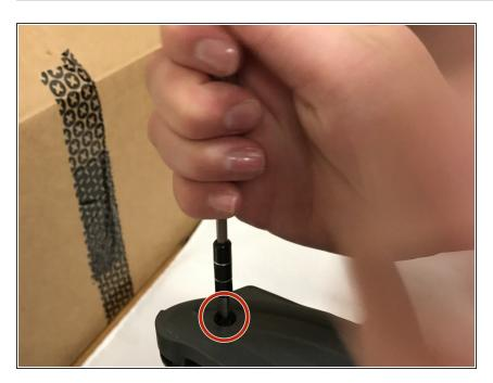
Use a T20 screwdriver to unscrew the 12.3 mm screw beneath the cover you just removed.
