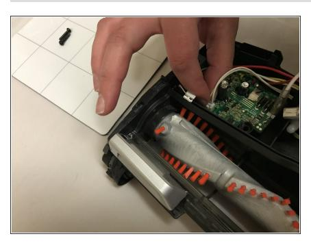
Squeeze tabs and remove small white plug with white and black wires coming out of it.
