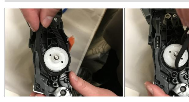
Pull the rubber brush roll band out of the large white gear.
