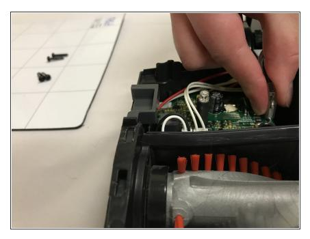
Remove the large black plastic plug using your fingers and/or long nose pliers.
