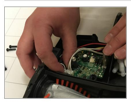
Squeeze tabs and remove small white plug with two white wires coming out of it.
