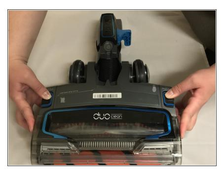
Press and slide the "access brush roll" buttons towards the text and lift plastic brush roll cover off.
