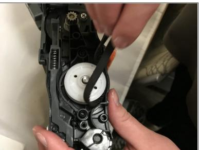
Pull the rubber brush roll band out of the large white gear.
