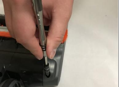
Move to the side of the casing with the shoe print mark. Use the T20 screwdriver to unscrew the 18mm screw.
