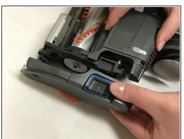
Use the small metal spudger to gently separate the side casing from the main body.
