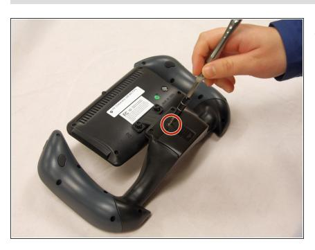
Using a JIS #0, unscrew the silver 4mm screw that holds the battery cover in place.
