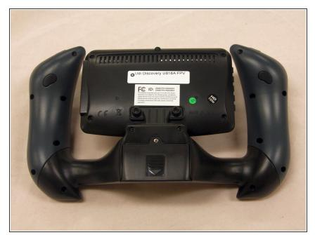
Turn the remote control over so that the buttons and joysticks are facing downward.
