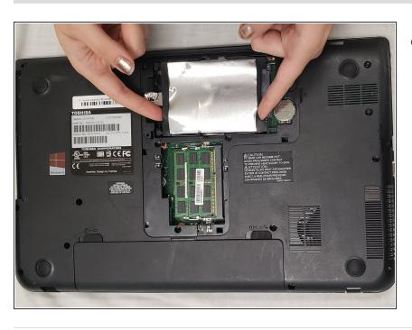
Carefully hold the sides of the hard drive with the rubber and pull the hard drive out. It should remove fairly easily.
