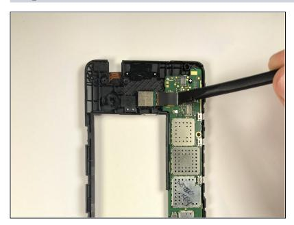
Using the pry tool lift up on the black tab
