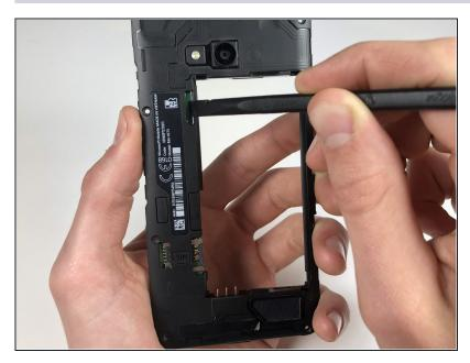
• Using the spudger, press out the motherboard.
