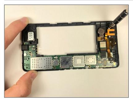
• Unscrew the 2 remaining screws with the T-4 bit.
