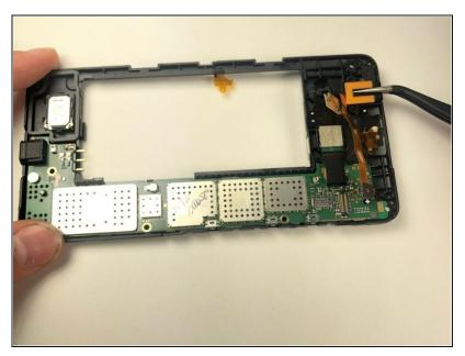
• Use the tweezers to remove the orange insulator foam.
