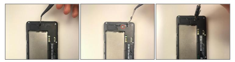
Use the <u>tweezers</u> to pull back the sticker, revealing the screw underneath.
