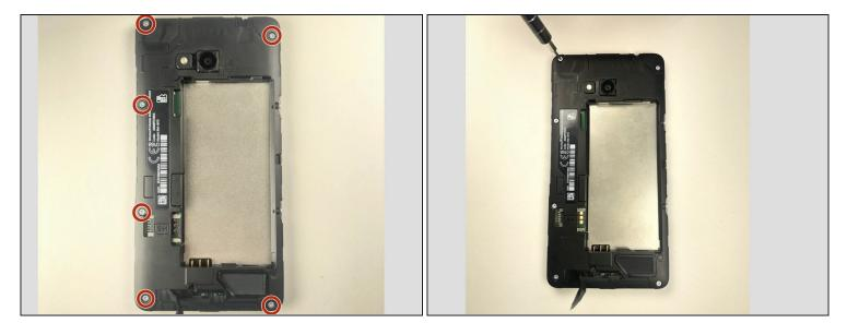
• Use a T4 Torx driver to remove the screws in the four corners, along with the two in the middle left side (six total).
