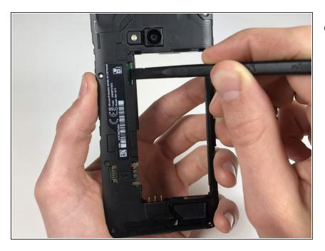
Using the spudger, press out the motherboard.
