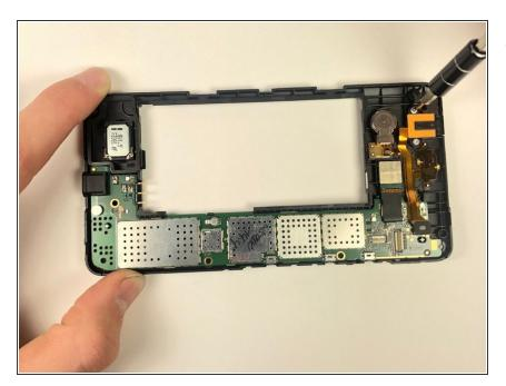
Unscrew the 2 remaining screws with the T-4 bit.
