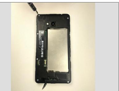
• Use a T4 Torx driver to remove the screws in the four corners, along with the two in the middle left side (six total).
