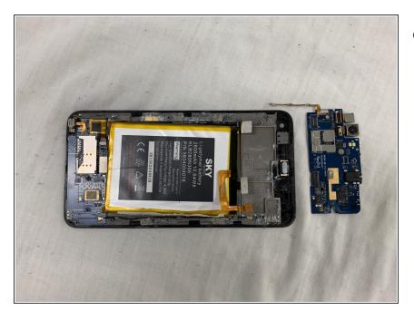
Once the screws are removed, gently lift the top motherboard and replace.
