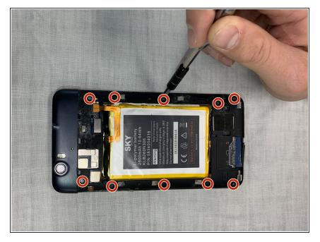
After removing back panel, remove all ten 3mm screws with the #00 Phillips screwdriver from the black plastic casing so it can be removed.
