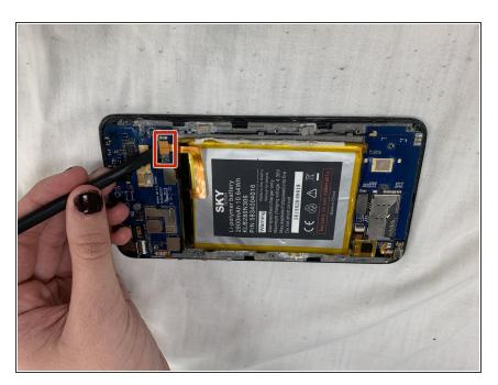
Use the spudger disconnect the gold cord extending from the battery to the top electronic board.
