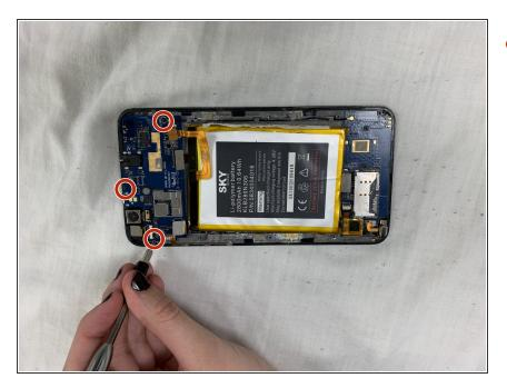
Use the #00 Phillips screwdriver to remove the three 3 mm screws attaching the top motherboard.
