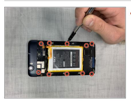
After removing back panel, remove all ten 3mm screws with the #00
