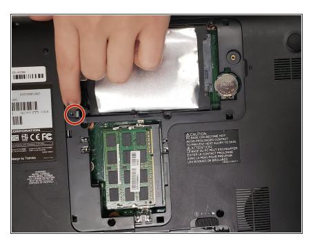
Under the back panel, remove the 4mm screw holding the disk drive in place.
