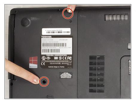
Remove the two 5-mm screws near the disk drive on the back panel.
