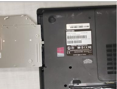
Carefully slide the optical drive out of its place in the laptop.
