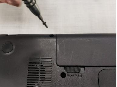
Unscrew the only screw (5 mm) that is holding on the removable back panel and remove the back panel.
