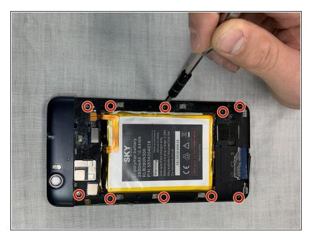
After removing back panel, remove all ten 3mm screws with the #00 Phillips screwdriver from the black plastic casing so it can be removed.
