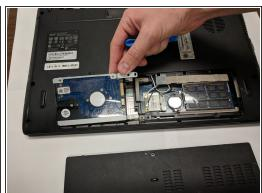
With a plastic opening tool slide the drive over and remove it.
