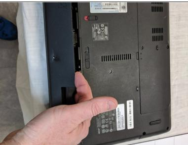
Place laptop upside down and push battery lock slider to the left to unlock. Lift battery out.
