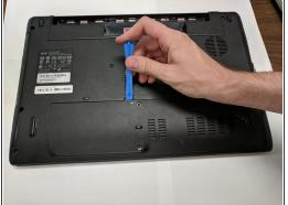
Remove two screws to take the cover off of the bottom of the laptop.
