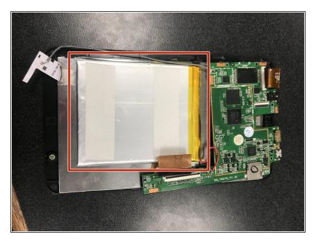
Look under the motherboard to find the battery. There will be yellow tape and black and red wires on the top of the battery.
