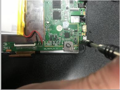
Find the third screw at top right corner below the USB port and use the same screwdriver from the previous two steps.
