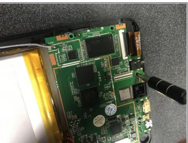
Find the second screw located above the white and grey box for the film for the camera and use the same screwdriver from step two to unscrew it.
