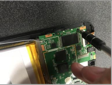
Find the first screw at the top left underneath the gold film and use a J0 Phillips Head screwdriver to unscrew it.
