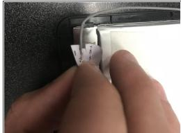
Carefully peel the sticker off the back of the screen sensor. DO NOT RIP THE STICKER!!
