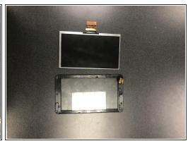
• Use the wedge from the camera replacement guide to go in between the silver lining of the Screen Sensor and Screen of the tablet.
