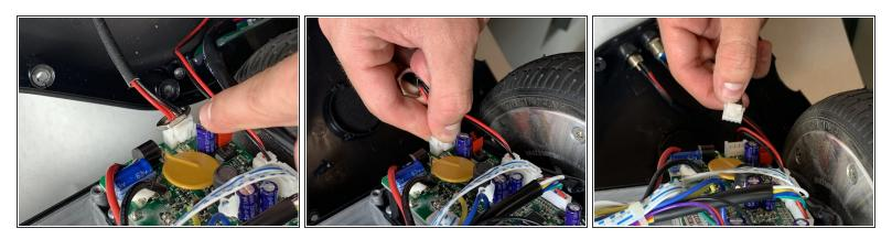
• Unclip the insulated red and black wires attached to the port from the motherboard
