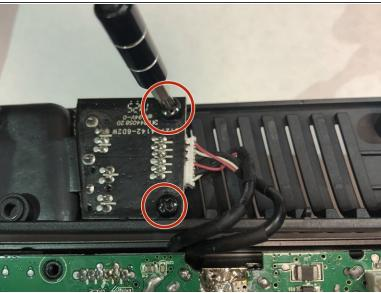
Remove the two screws using the Phillips #1 screwdriver. Once they are unscrewed, the panels will hang loose allowing unobstructed access to the motherboard.
