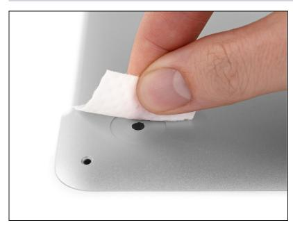
Scrub the foot cavity with adhesive remover to remove any remaining adhesive.
