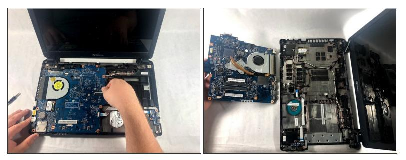
• Gently lift and remove the motherboard off of device.
