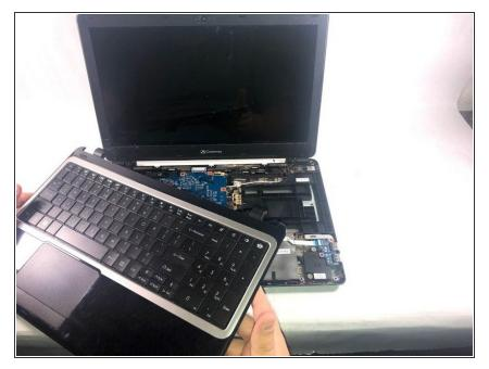
• Lift the upper case cover off of the device. Use a prying tool along the edges if necessary.
