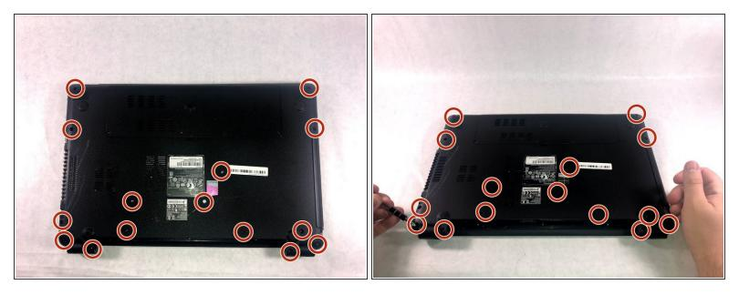
• After removing the battery, remove 15 7mm screws using the Phillip #1 Screwdriver.
