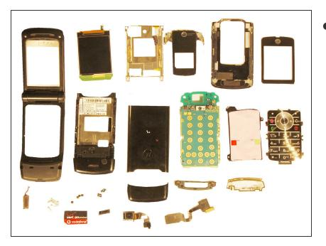
From left to right, top to bottom: Outer Casing, LCD Screen, Upper Metal Frame, Outer LCD cover, Upper Cover, Inner LCD Cover, Lower Metal Casing, Back Casing (Upper), Lower Circuit Board, Keypad, Keypad Membrane, Speaker, Screws, Screw Covers, Back Casing (Lower), Upper Casing Support, Circuit Board Support, SIM Card, USB cover, Camera, Flex Cable
