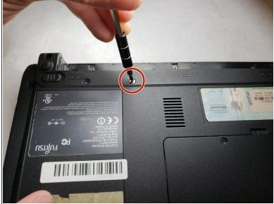
Remove the two 3 mm PH0 screws holding hard drive in place.
