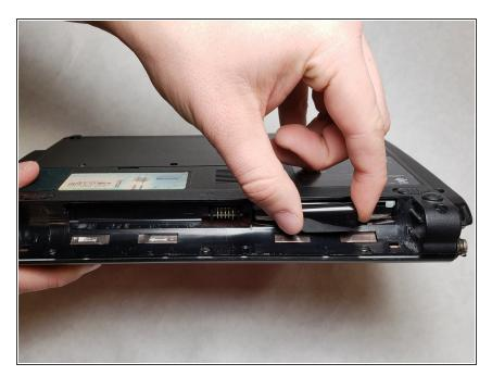
Unfold the black tab attached to hard drive.
