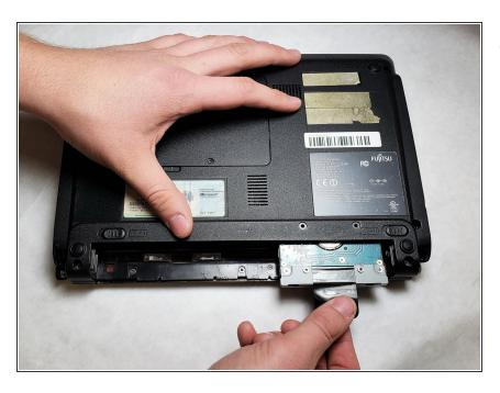
Remove the hard drive by pulling the black tab.
