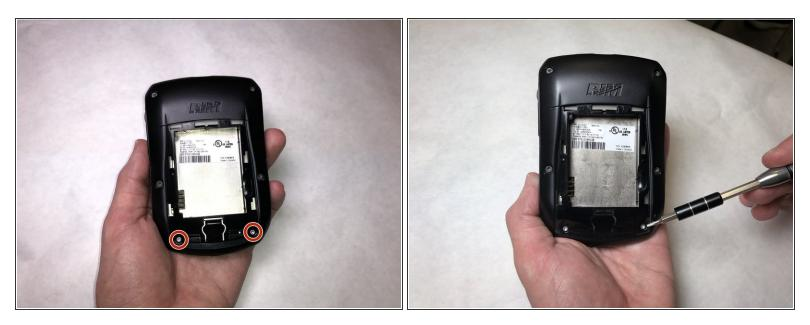
• Remove the two 5 mm Torx T6 screws.
