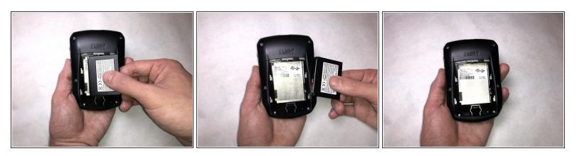
• Remove the battery from the compartment.
