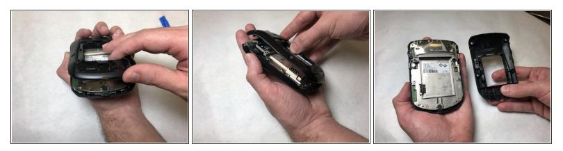
• Grab the back housing from the bottom and lift the housing away from you.
