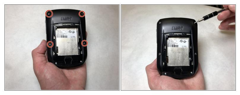
Remove the four 10.7 mm Torx T6 screws.
