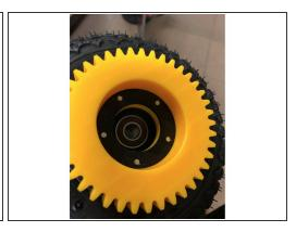
• Use 5 x M4 bolts to attach wheel gear to the wheel hub for gear meshing.
