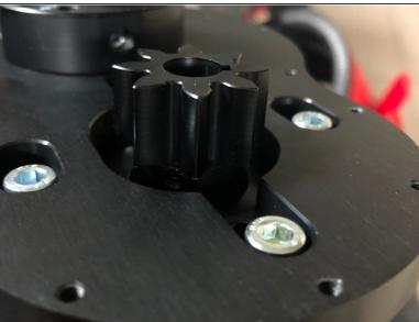
Use provided 4 x M3 bolts to attach motor (with motor mount adapter if use)
