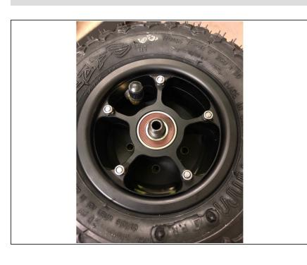
Make sure 5 x M4 bolts are tighten securely.
