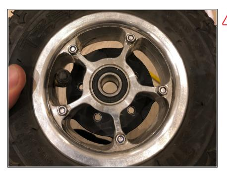
Make sure to tighten nuts in star pattern to make sure equal tension on all bolts
