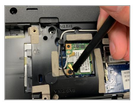
Dislocate the black wire by pushing upward away from the network card.
