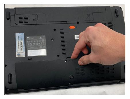
Lift and remove the cover panel via the indentation in the middle of the panel.
