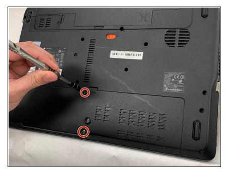
Unscrew the two 7 mm long #0 Phillips screws.
