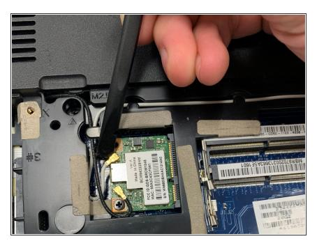
Dislocate the white wire by pushing upward away from the network card.
