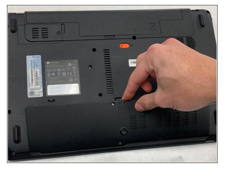
Lift and remove the cover panel via the indentation in the middle of the panel.
