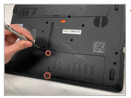
Unscrew the two 7 mm long #0 Phillips screws.
