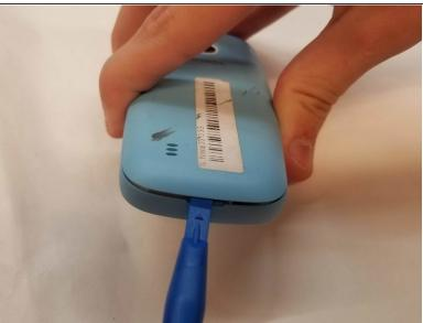
Using the thumbtab molded on the bottom of the phone, pry the back cover off using either a fingernail or a plastic opening tool.
