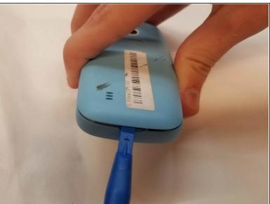
Using the thumbtab molded on the bottom of the phone, pry the back cover off using either a fingernail or a plastic opening tool.
