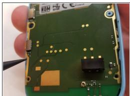
Use a spudger to simultaneously leverage the shell away and the motherboard up from the body of the shell.
