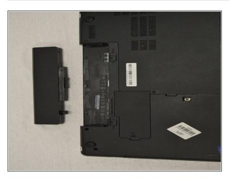
Remove the battery from the device.
