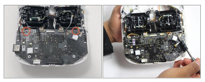
• With the Phillips #00 screwdriver, remove the two Phillips screws.
