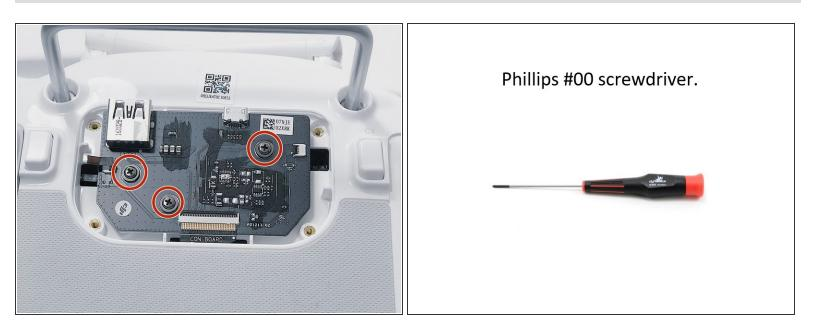
Remove three screws using a Phillips #00 screwdriver.
