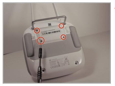
Remove the four screws with a Torx T8 screwdriver to access the back con board.
