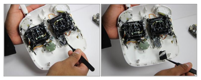
• Carefully remove the plastic. This will help you gain access to the power button panel.
