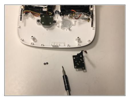
Gently pull the power button out from the panel. Replace it with a new one.
