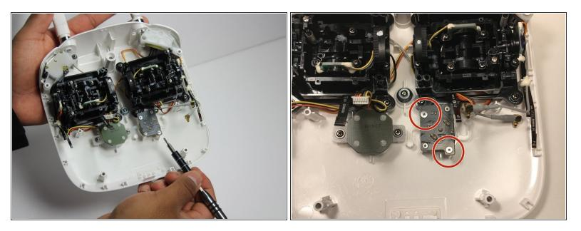
With a Phillips #00 screwdriver, remove the two screws on the power button panel.
