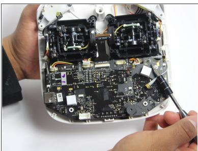
With the Phillips #00 screwdriver, remove the two Phillips screws.
