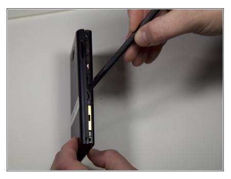
• Begin by using the nylon spudger to pry off the back case.
