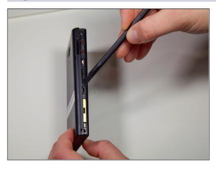
• Begin by using a nylon spudger to pry off the back.
