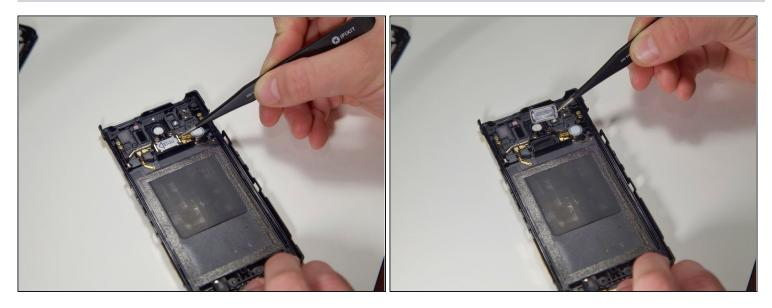
• On the back cover of battery casing, remove the speaker using the <u>tweezers</u>.
