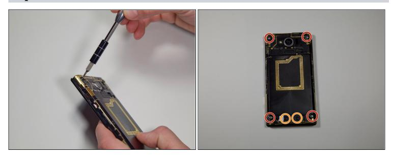
• Remove case around battery using a T5 screwdriver to remove four 5mm silver screws.
