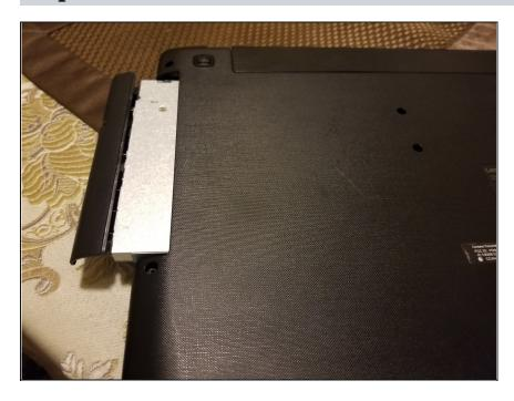
• Remove the screw that is under the two keyboard screws and pull the disk drive out.
