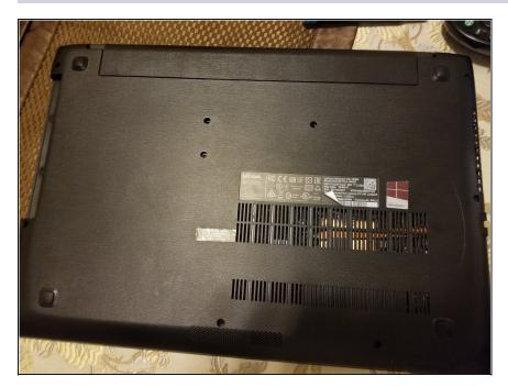
• Remove all of the screws on the outside edge of the bottom.
