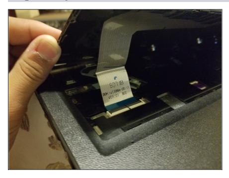
• Remover the ribbon cable and remove the keyboard afterward.
