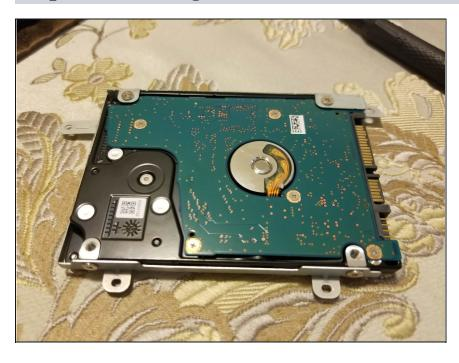
• Remove the four screws the hold the metal cage onto the drive to separate them.
