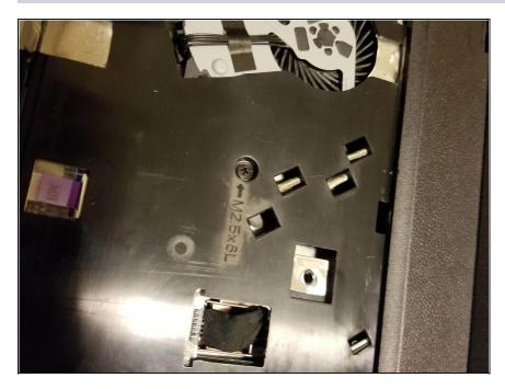
• After the keyboard is removed, remove the screw and the battery connector.
