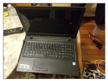
• Insert a prying tool in the crack between the keyboard and frame. Start by the power button and go all the way round the keyboard.
