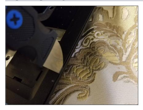
Flip the laptop over and in the crack between the two case pieces slide a prying tool in between and follow the perimeter until the two pieces are separated.
