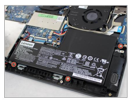
Using the JIS #0 screwdriver unscrew the three battery screws.
