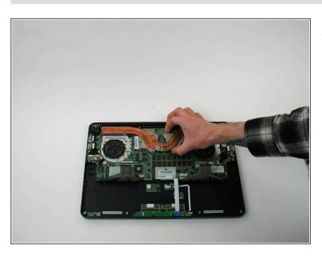
Lift the cooling rod straight up and out of the laptop.
