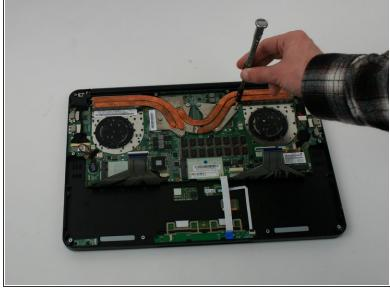
Using a Phillips #0 screwdriver, remove the six 8 mm screws holding the cooling rod to the motherboard.
