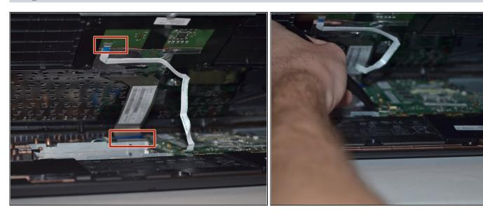
• Lift palm rest and unplug keyboard cable and touchpad cable using tweezers. After these two cables have been unplugged you can remove the keyboard cover panel.
