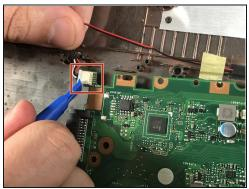
• Flip the motherboard over and use the plastic opening tool to unplug the black and red wires from the motherboard.
