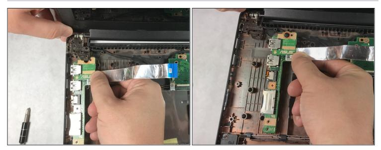
• Slightly pull the unhinged screen up to free the board and remove it.
