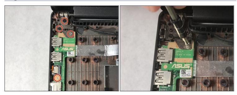
• Locate the I/O board on the left of the computer. Using the Phillips #0 screwdriver, unscrew the three 5mm screws to unhinge the screen, which will free the board allowing it to be removed and replaced.
