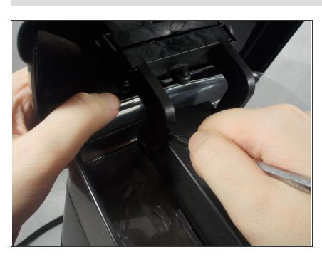
Repeat the last step on the other hinge, making sure to keep a firm grasp on the lid as it comes off to avoid dropping it.
