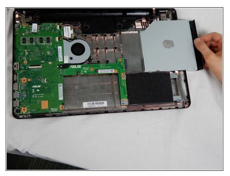
• Slide the disc drive to the right, removing it from the laptop case.
