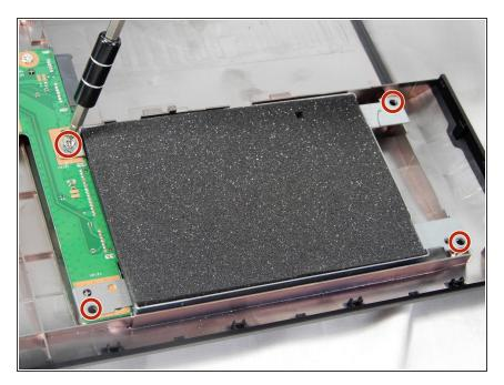
Using the Phillips #0 screwdriver, unscrew the four (5.7cm) screws around the hard drive.
