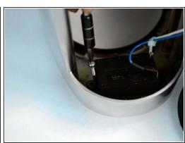
Remove two 11.59mm T10 screws.
