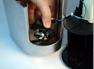
Remove the time/on switch by pulling upwards.
