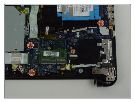
Using a Phillips #00 screwdriver, remove the three 3 mm screws on the board with white arrows pointing to them.
