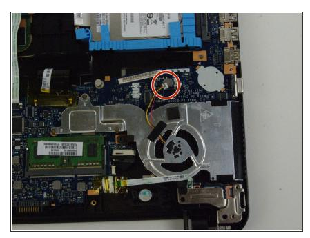
Disconnect the fan wire from the motherboard.
