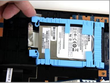
• The hard drive is held in place with a soft, blue rubber retainer. The retainer can be disconnected by pulling up on the two tabs at the left side of the hard drive in these images.
