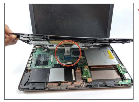
Lift the plastic cover and unplug the three data cords (not all pictured) under the cover from the keyboard and motherboard.
