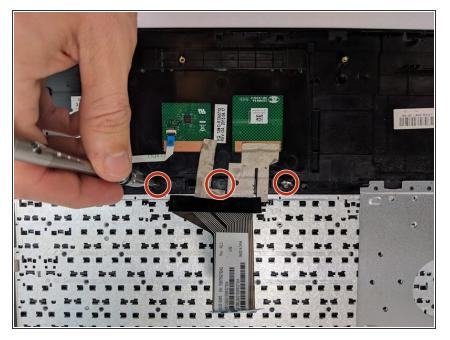
Locate and unscrew the three 3.2 mm at the top edge of the touch pad using the Phillips #0 screwdriver.
