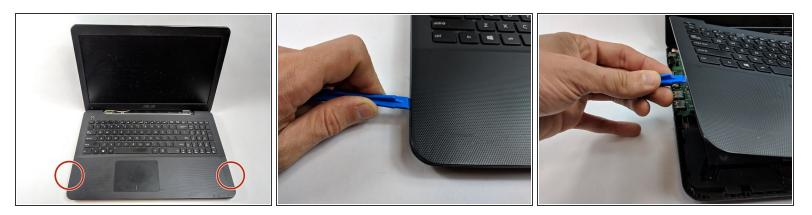
Once the screws are removed, carefully lift both sides of the plastic keyboard/touch pad cover with a plastic opening tool.
