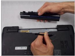
While the battery release switch is pushed to the right, carefully slide the battery out of its socket.
