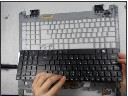
Use the metal spudger to lift the keyboard component out of the metal panel.
