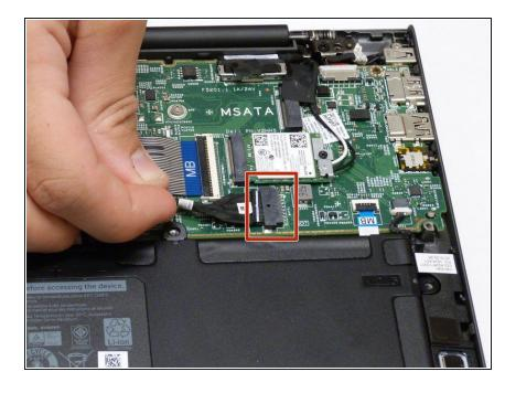
Use your fingers to remove the connecting cable to the battery unit.
