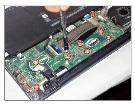
• Remove the eight 2mm screws securing the motherboard in place.
