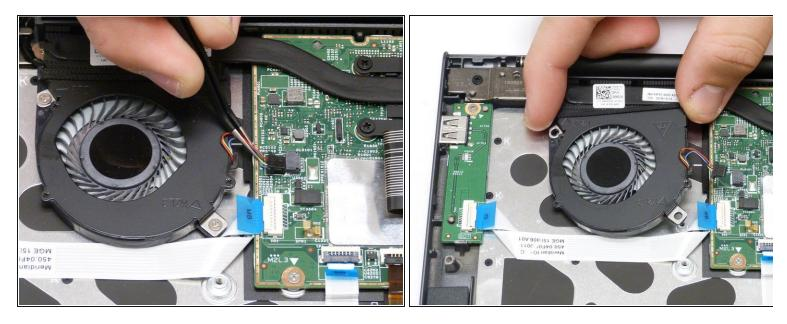
• Using your fingernails, pull the cooling fan cables loose from the motherboard.
