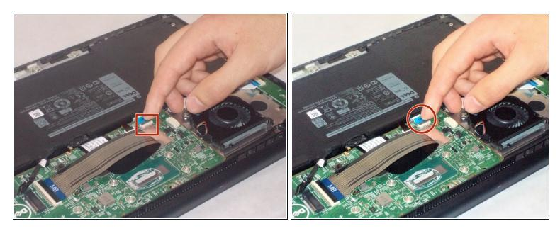
• Pull up on connector tab to release touchpad cable.
