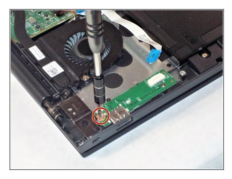
Remove the single 2mm screw securing the IO board to the laptop.
