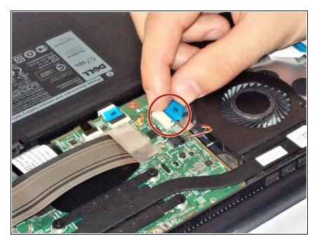
• Pull up on connector tab to release IO board cable.
