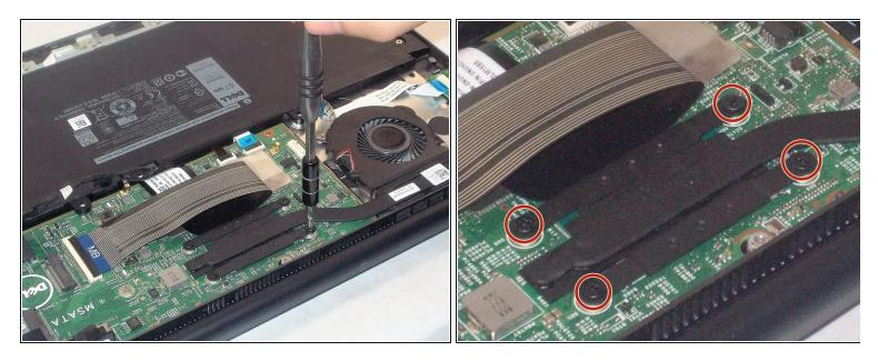
• Remove 4 screws securing heat sink.
