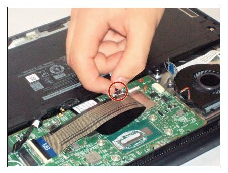
• Release the keyboard backlight cable.
