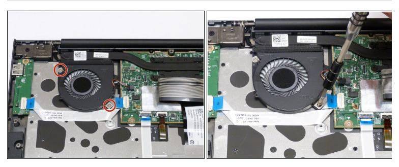
• Using the #1 Philips screwdriver, remove the two, 2mm screws securing the fan assembly.
