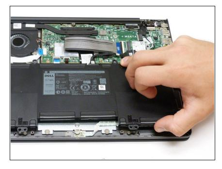
• To remove the battery, lift up on one side to get your fingers underneath and lift away.
