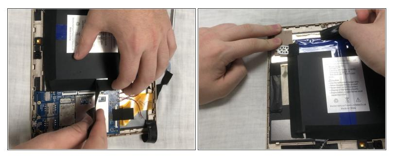
• Remove electrical tape placed around the battery to keep it in place.
