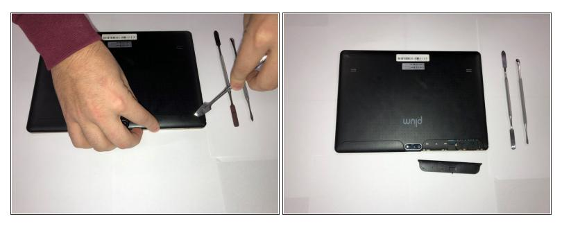
• Use a metal spudger to remove the small panels to the immediate left and right side of the camera.
