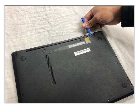
Use the iFixit opening tool to pry off the back cover of the laptop.
