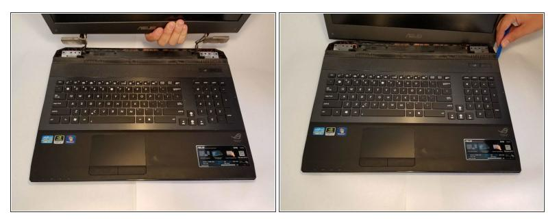
• With the screen removed, pry the piece that has the keyboard and the track pad on it.
