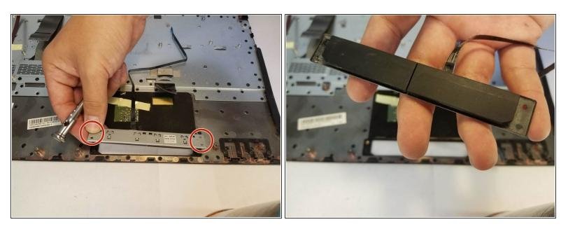
• Remove the two Phillips head screws holding the buttons in place.
