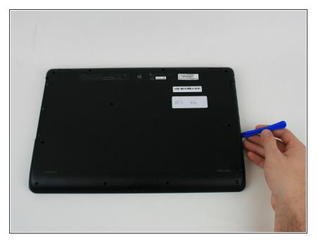
• Run the opening tool along the bottom cover seam.
