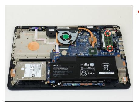
Locate the two metal clips securing the RAM.
