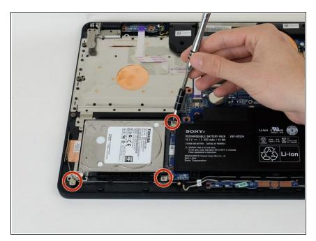
Unscrew the three 4mm screws with the Phillips #0 screwdriver located on the outer edge of the hard drive.
