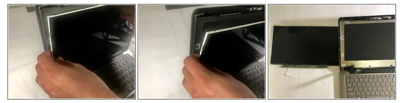
Remove the screen by grabbing the edges of the screen and pulling forward.
