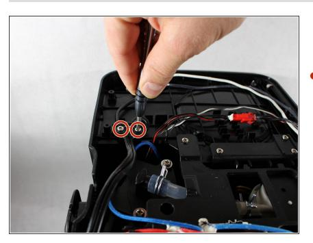
Loosen two 6mm #1 Phillips head and remove clamp holding power cable.
