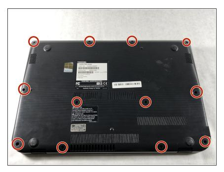
Remove the twelve 5 mm Phillips #1 screws from the back panel.
