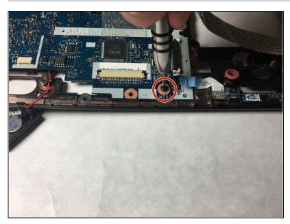
Remove the 3mm #00 Phillips screw near the bottom of the blue board.
