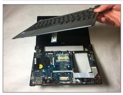
• Lift the keyboard off of the back casing.
